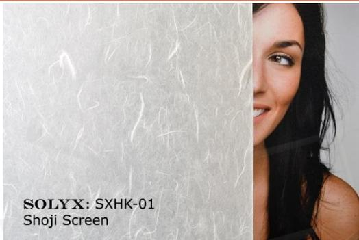
SOLYX® SXHK-01 Shoji Screen film is recommended for application to interior and exterior glass (inside surface). Made of durable Polyester fiber and PVC combination with a decorative surface. Total nominal thickness is 4 mil. Supplied with a silicone liner, which protects the clear, pressure-sensitive adhesive, and applied using the same tools and techniques for window films.
